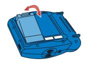
Initiate AED selftest by re-inserting battery
